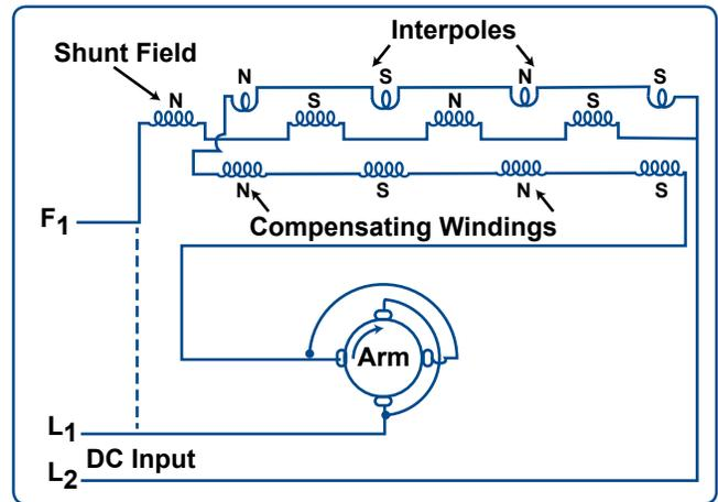
Figure 2. Interpole circuit.
