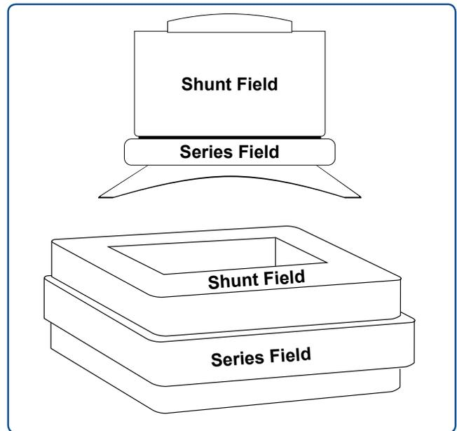
Figure 3. Stab shunt and compound coils.
